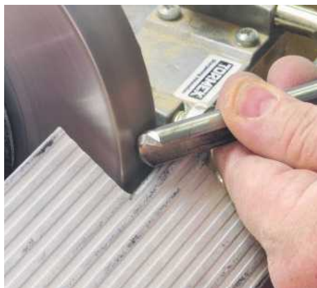
▲ Pic.2 The heel of the tool is ground off by resting the tool on the toolrest with the flute pointing towards you. This will stop you rubbing too much bevel on the workpiece and over-compressing the timber
